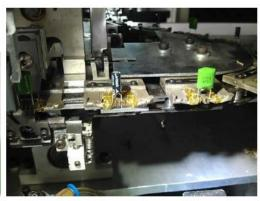
Tooling to accommodate a variety of applications-field reconfigurable Single Span: 2.5mm Dual Span: 2.5mm/5.0mm Triple Span: 2.5mm/5.0mm/7.5mm
